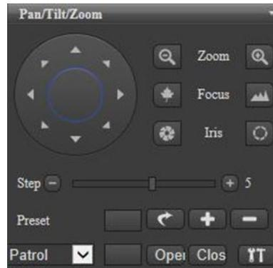
Figure 4. PTZ control panel
