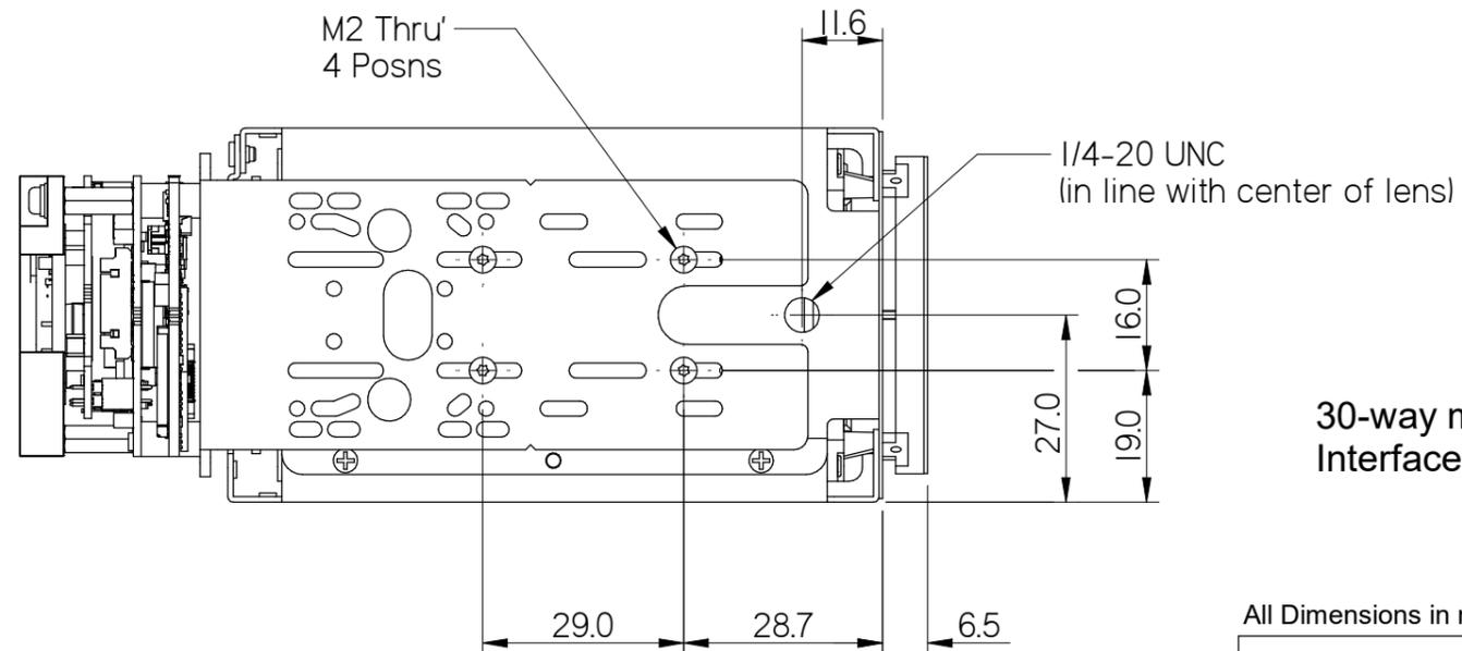
30-way micro-coax - Camera to Interface Board cable - not shown
