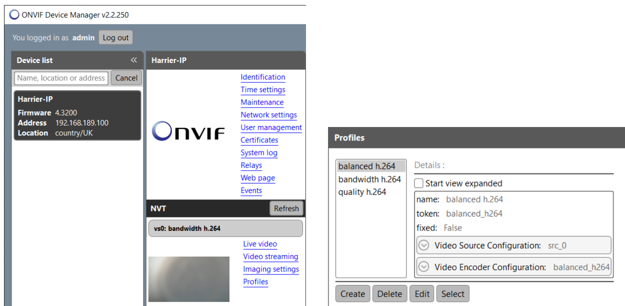
Figure 18. ONVIF Device Manager main menu and Profiles window
