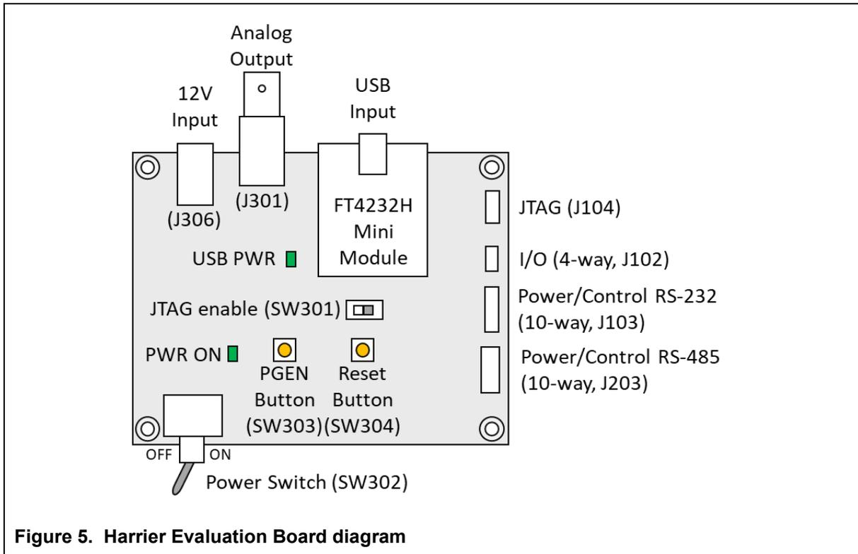
**Figure 5. Harrier Evaluation Board diagram**
