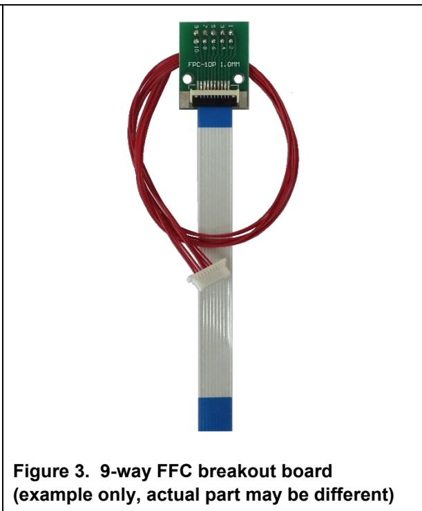
Figure 3. 9-way FFC breakout board (example only, actual part may be different)
