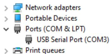
**Figure 6. Typical Harrier HDMI 4K camera COM port in Device Manager**
